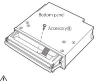
Never insert the screw in any other screw hole than the one specified. If you screw them in another hole, it will contact and may cause damage to the mechanical parts inside the unit.
